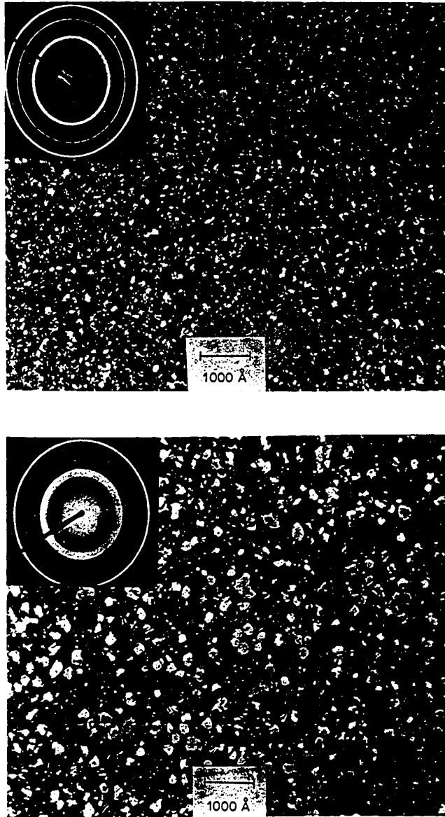
Fig. 3-6: (a) Transmission electron micrograph and diffraction pattern for a 300 Å Ta film on a 30 Å Nb underlayer to nucleate the bcc crystal structure. (b) Same as (a) but without the 30 Å Nb underlayer. This film has the \beta -Ta (tetragonal) crystal structure. (both (a) and (b) were deposited on a 200 Å carbon film on a standard 200 mesh TEM grid.
