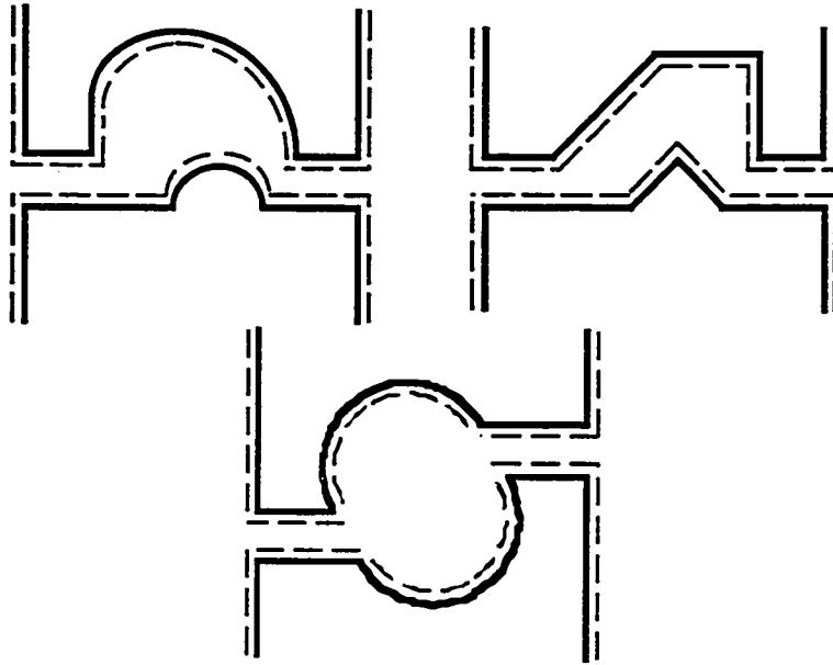
Figure 6.5 Scale drawings of the cavities of sample MBE17S9 showing the edges of the etched mesa as solid lines and the edges of the electron gas with 85 nm of depletion as dashed lines. There would also be significant rounding of the corners which is not shown in these drawings. The solid lines are based on the scanning force microscope images of Figure 4.6.
